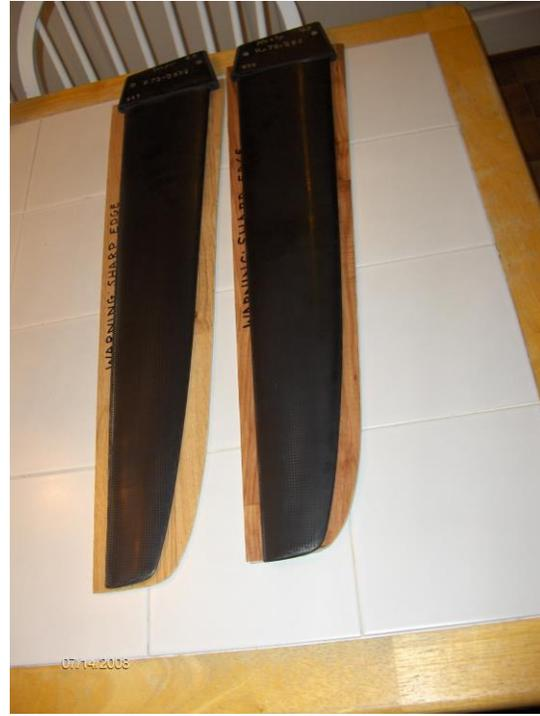
Photo 1c. Two "cut" fins with the 2008 tip shaping.
